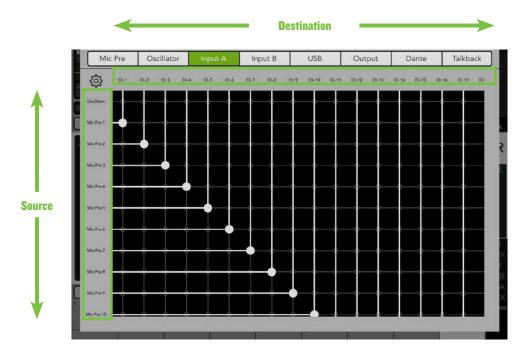
The source and destination may change, but the default patching for each channel input A is mic pres 1-xx routed to channels 1-xx and USB 1-2/4 routed to returns 1-2/4. Additionally, mic pre 16 [DL16S] / 32 [DL32S, DL32R] is routed to talkback. Drag anywhere in the black box to view these other routings.
