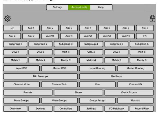
With no access limits buttons pressed, the device can access all controls. With one or more buttons pressed, the corresponding control will be hidden and cannot be accessed or changed from that device. The function of the limiting buttons is described below.
