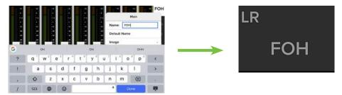
As seen in all of these images, a small name resides in the upper-left corner of the master ID button regardless of the name and/or image. This system name represents each output and it cannot be changed or removed. Trust us, it's for the best, as it is for easy identification of each output, even after you rename it something goofy.
