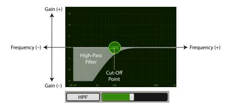
**High-Pass Filter (Disengaged)**
