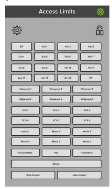
Check out the two images below. On the left side, we set access limits to everything except aux 1. On the right hand side is an image of the mixer view with the above-mentioned access limits in place. Notice that only the Aux 1 functions are accessible. Also, on the far right, Aux 1 is the only available output and the output selector can't even be opened. Other than that, nothing but darkness exists.
