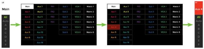
Once a different mix has been selected, the color surrounding the channel faders will change to show the newly selected output. Similarly, the master fader will display the newly selected mix. In this case, LR to A4.
