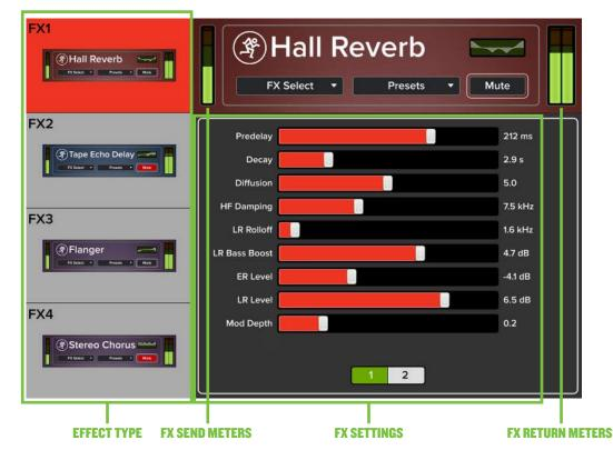
**FX Send Meters** — There are separate vertical send meters, one for each effect.
