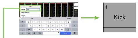
Before moving on with the rest of the Channel ID, let's look at another exciting feature regarding channel naming. On the left and right side of Name: are "previous" and "next" arrows<sup>5</sup>. This makes it easier to edit the names of multiple channels in a row without having to re-tap each channel's ID button just to name it.
