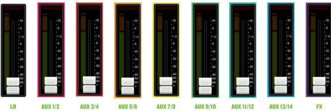
Notice how each channel's input meter is surrounded by the color of the selected output. In the left image, the faders control the levels going to the LR mix, while the faders on the right image control the levels going to the aux 1 mix. As seen in the images below, all we did was change the selected output from main LR to aux 1.
