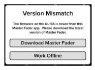
Master Fader App Needs an Update The Master Fader app automatically compares the app and firmware versions each time the app connects to the mixer. In order to operate properly, the firmware and app versions must match. If the Master Fader app is older than the firmware version in the mixer, you will be prompted to update the app. Tap the 'Download Master Fader' button on the popup and update as described on the previous page.
