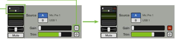
**48v Phantom Power Disengaged**
