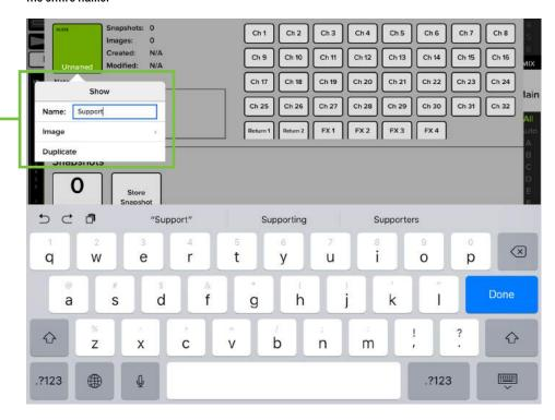
The shows button displays the name of the last recalled snapshot. In this case it is the default "Shows". If an asterisk \* is displayed, this lets you know that the state of the console has changed (whether the shows panel is open or not).
