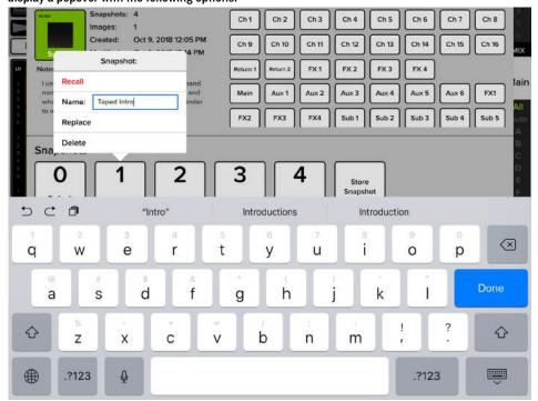
Tap inside of the blank "Name:" box to reveal the onscreen keyboard, then name the currently selected snapshot as you so desire. Tap the blue "Done" key when satisfied with the name. If the name is too long to fit, the button scrolls, displaying the entire name.
