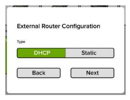
**DHCP** — DHCP stands for Dynamic Host Configuration Protocol. In short, the external router needs to be able to assign an IP address to a device – i.e. one of the DL mixers – connected to the Ethernet port. This is the most common selection, with the IP address changing (automatically) being assigned automatically by the external Wi-Fi router each time it connects. More information and screen shots on the following page.
