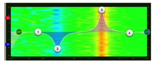
The RTA / spectrograph is available on all channel inputs and outputs. There is only one instance of the RTA implemented in the mixer. Therefore, only one channel can show the RTA or spectrograph at a time regardless of how many devices are connected.
