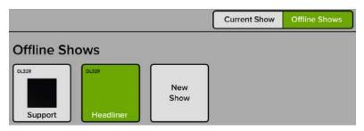
As stated on the Load Show popover, the load time is all dependent on the number of stored snapshots on the show. It can take up to two seconds per snapshot and 30 seconds per image to transfer. The current state of the console is not changed on a show load, audio still passes and you can still adjust all mix controls. However, in reality, you will probably want to wait to recall a snapshot from the new show after loading the show completes.
