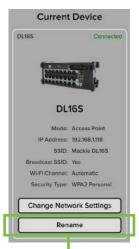
**Change Network Settings • Rename** — When a device is connected to a mixer (either wired or wirelessly), you are able to set up some advanced configuration settings for the mixer. Two buttons are located in the Current Device box: Change Network Settings and Rename.
