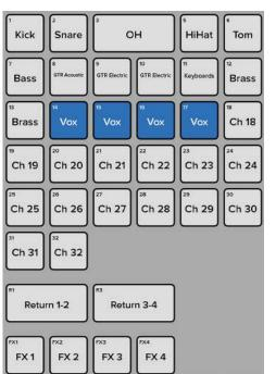
To route signals to a subgroup, tap a subgroup's routing button followed by tapping the button of every channel that should be a member of that subgroup. Assigned buttons will illuminate, while unassigned channels will remain gray. It is permissible for any channel to be a member of multiple subgroups. In this example, we're sending channels 14-17 [lead and background vocals] to subgroup 1.
