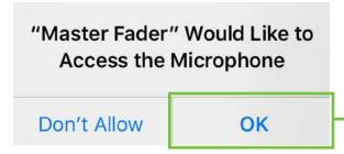
Even though Master Fader does not use the microphone to record, you need to approve this request in order to allow it to record over the dock connector. If you don't allow access, Master Fader will record short, empty audio files.
