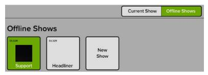
At this point the show has been created, but it is still an Offline Show. It has to be the Current Show in order to view and load snapshots. That's easy! Just tap the Headliner button to reveal a popover similar to what is displayed at the top of this page. From there tap the red Load button to reveal an image similar to what may be seen below.
