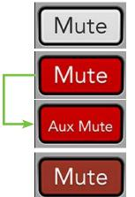
**Mute** – Mute buttons do just what they sound like they do. They mute – turn off – the signal on the channel(s). Engaging a channel's mute switch provides the same results as sliding the channel fader all the way down.
