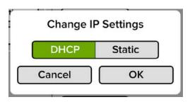
**DHCP** — DHCP stands for Dynamic Host Configuration Protocol. In short, the external router needs to be able to assign an IP address to a device – i.e. one of the DL mixers – connected to the Ethernet port. This is the most common selection, with the IP address changing (automatically) each time it connects. More information and screen shots on the following page.
