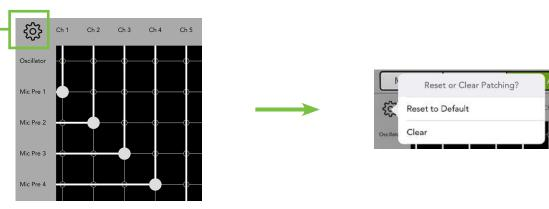
Reset to Default resets (the currently opened tab) to its default state. Clear clears all patchings (of the currently opened tab) and all balls will be removed from the I/O patch. Clearing all routings may be used in more complex setups where it's easier to start from scratch. Once cleared, the source(s) and destination(s) may be tapped into spot for your needs.
