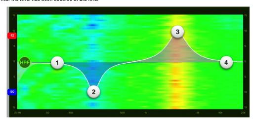
The RTA / spectrograph is available on all channel inputs and outputs. There is only one instance of the RTA implemented in the mixer. Therefore, only one channel can show the RTA or spectrograph at a time regardless of how many devices are connected.
