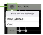
From here you can choose to reset the I/O patch to its default or clear the routing.
