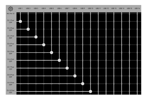
**OUTPUT 1** — Perhaps the mixer will be used strictly as a monitor mixer with no need for main L/R. Here you're able to use all outputs as linked aux sends for a total of seven in-ear and/or 14 wedge monitors.
